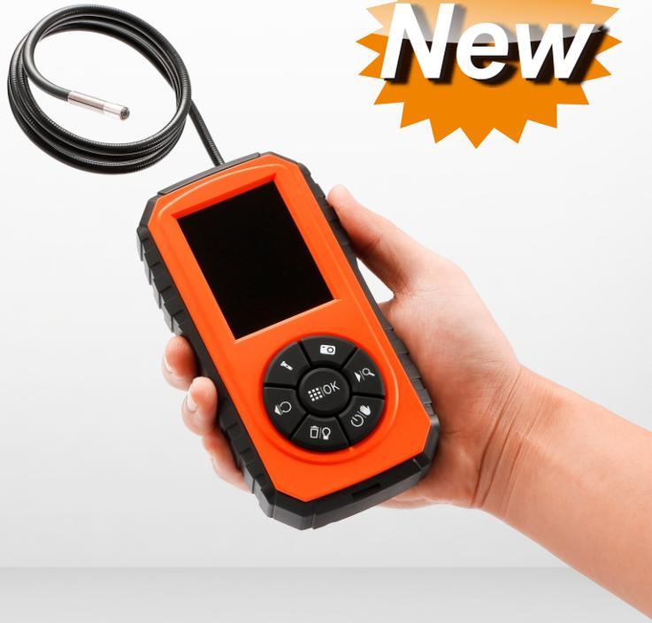
The PocketScope is a real pocket-size endoscope camera with its 1m camera tube wound inside the back part of the product. Featured with 5.5mm semi-flexible tube, HD 720P resolution, SD card recording, etc; It's a great tool for inspecting hard to reach areas.
