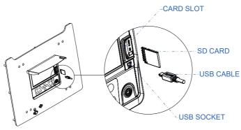
Figure 14. Install SD Card
