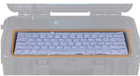
The system comes with a keyboard which you can use it to write simple notes on the screen and this will be displayed on the images and videos that are stored in SD card.
